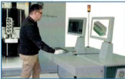
User friendly CT operation and evaluation, e.g. automated wall-thickness measurements on a scanned cylinder head
