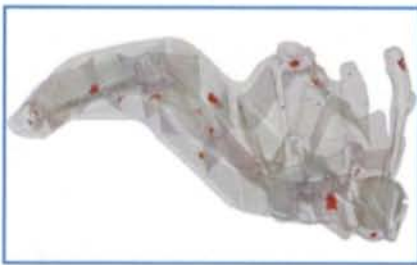
Automated 3D porosity analysis in an automotive control arm
