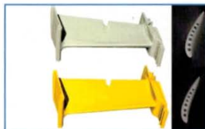
Up to 300 kV high power scans (below) ensure reduced artifacts e.g. for turbine blade inspection tasks
